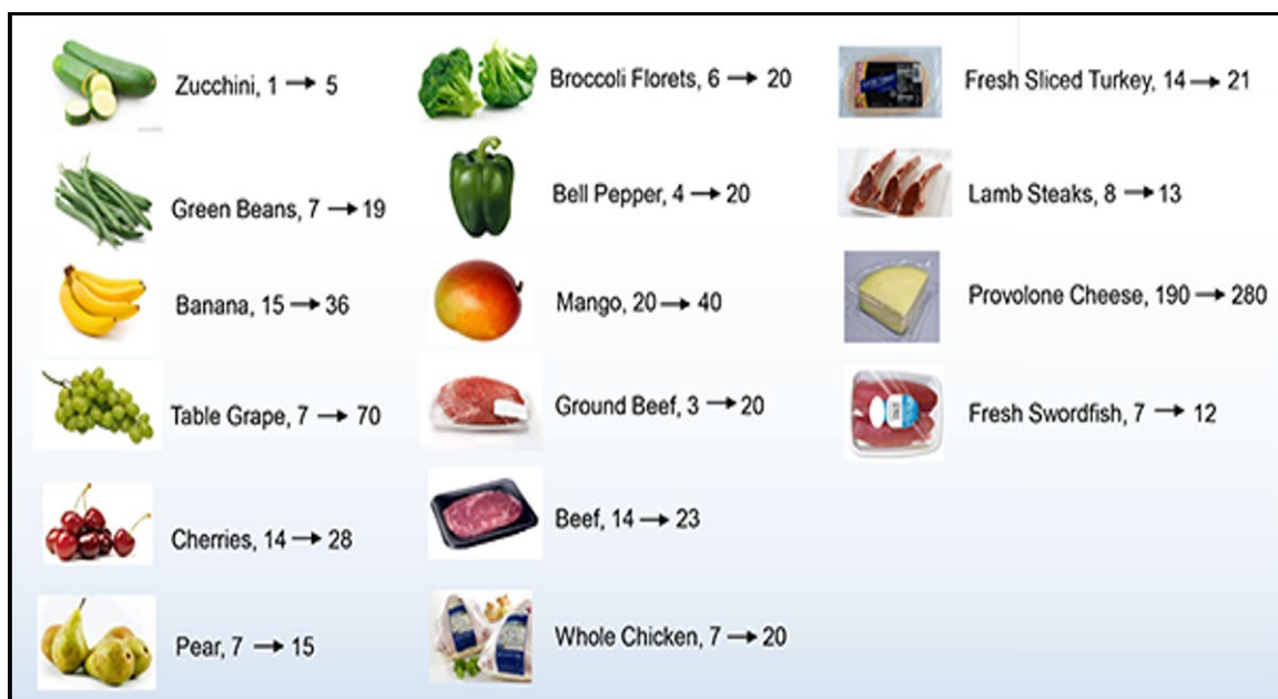
Figure 1 – Comparison of the Shelf Life of Selected Grocery Items without Flexible Packaging (in days) and with Flexible Packaging (in days)
