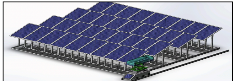
SolarACM's Kolchar S2 slides along a track to clean solar panels.
